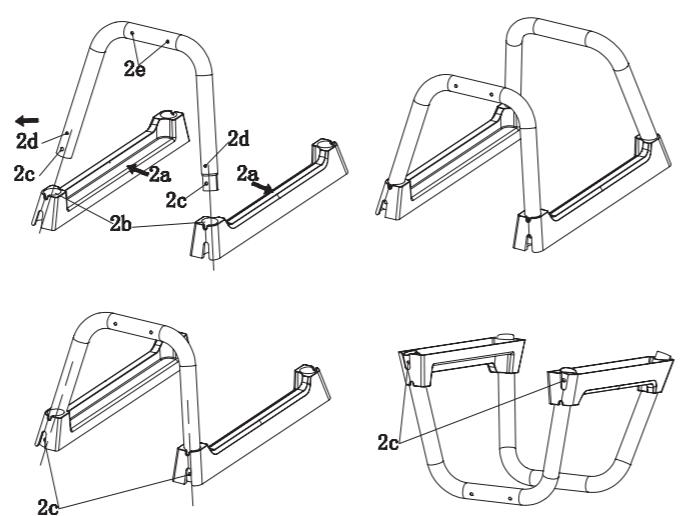
Insert the straight tube (11) with shrinkage side into the hole of the U-shaped tube (10) without shrinkage side.
